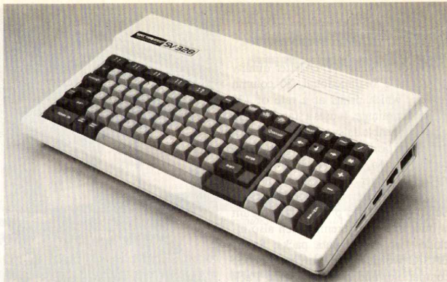
Spectravideo's new SV-328 personal computer features an 87-key full stroke keyboard along with built-in 48K ROM and 64K user addressable RAM.
